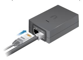
5. Connect the *Power Cord* to the power port on the *airFiber PoE Adapter*. Connect the other end of the *Power Cord* to a power source.
