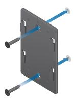
Attach the airFiber PoE Adapter to the bracket by aligning the four slots and tabs, and then slide the adapter downward.
