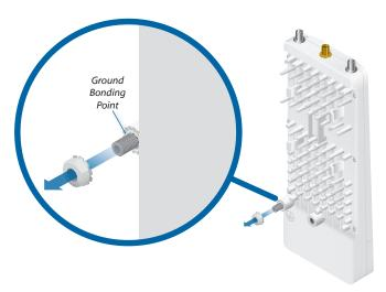
2. Attach a ground wire (min. 10 AWG or 5 mm²) to the lug and replace the nut to secure the wire.
