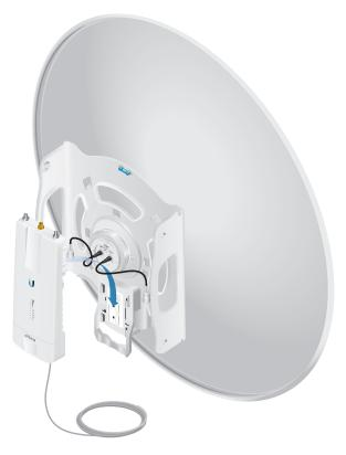
2. Attach the RF cables from the antenna feed to the RF connectors on the airFiber X radio in this combination: +45° to Chain 0 and -45° to Chain 1.
